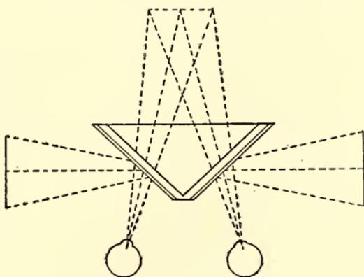
FIG. 49. Plan of Wheatstone's Stereoscope.
