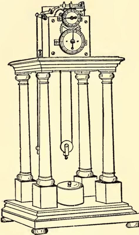
FIG. 62. Hipp's Chronoscope, an electrical clock whose unit is  $\tau$ : commonly employed in the reaction experiment.
